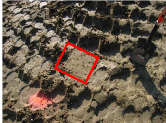
(b) Test depth at bottom of padfoot penetration.
