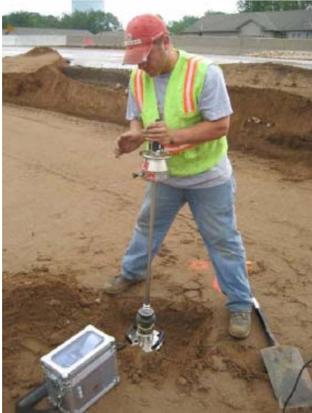
(a) Test depth at one-half the lift thickness.
